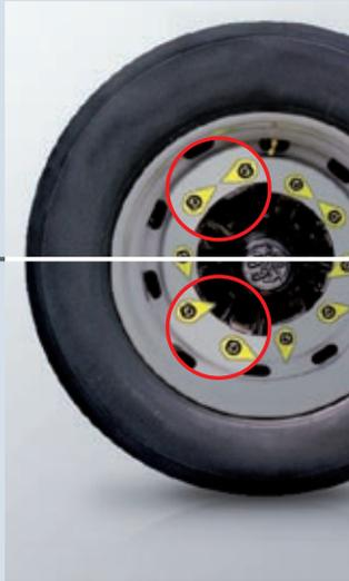
Any movement of the wheel nut will be clearly evident.
